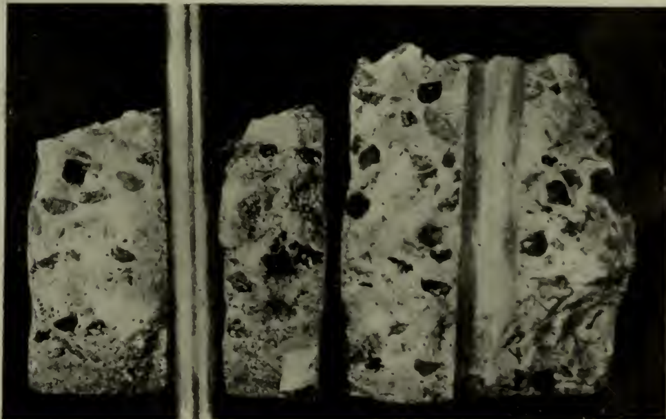
FIG. 1. SLAG CONCRETE AFTER SIX YEARS' EXPOSURE TO WET CONDITIONS, BROKEN TO SHOW STEEL BRIGHT. The part of the Bar outside the Concrete is shown in Fig. 2.
